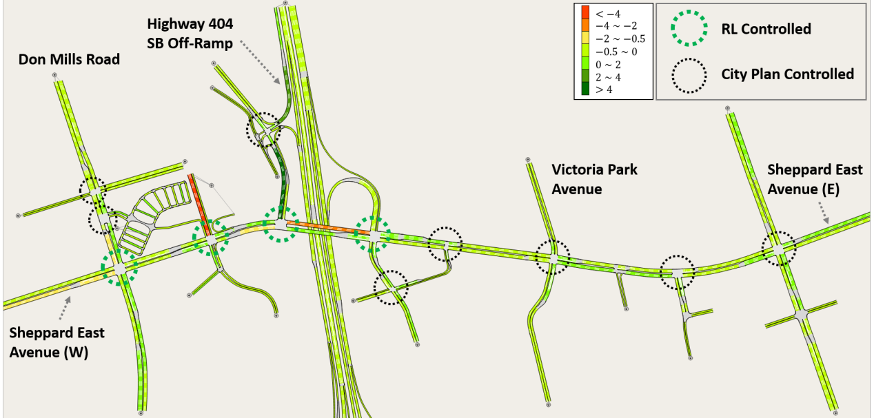
FIGURE 11: The heatmap of queue difference between the City Plan and our RL approach with 3-hop upstream setup. The road-wise comparison is based on the average queue length over the whole simulation time. Roads labeled in green indicate improved queue length in our approach compared to the City Plan, while roads in red indicate longer queues.
